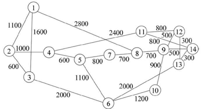
Fig. 3. NSFNet topology with 14 nodes and 21 bidirectional links (distances measured in kilometers).
