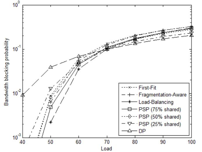
Fig. 4. Comparison of bandwidth blocking probability in logarithmic scale.
