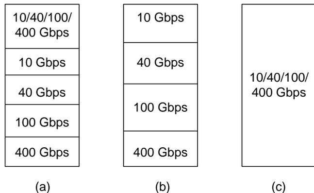
Fig 2. Partial-sharing partitioning (PSP) with different percentages of shared spectrum: (a) 25%, (b) 0%, and (c) 100%.
