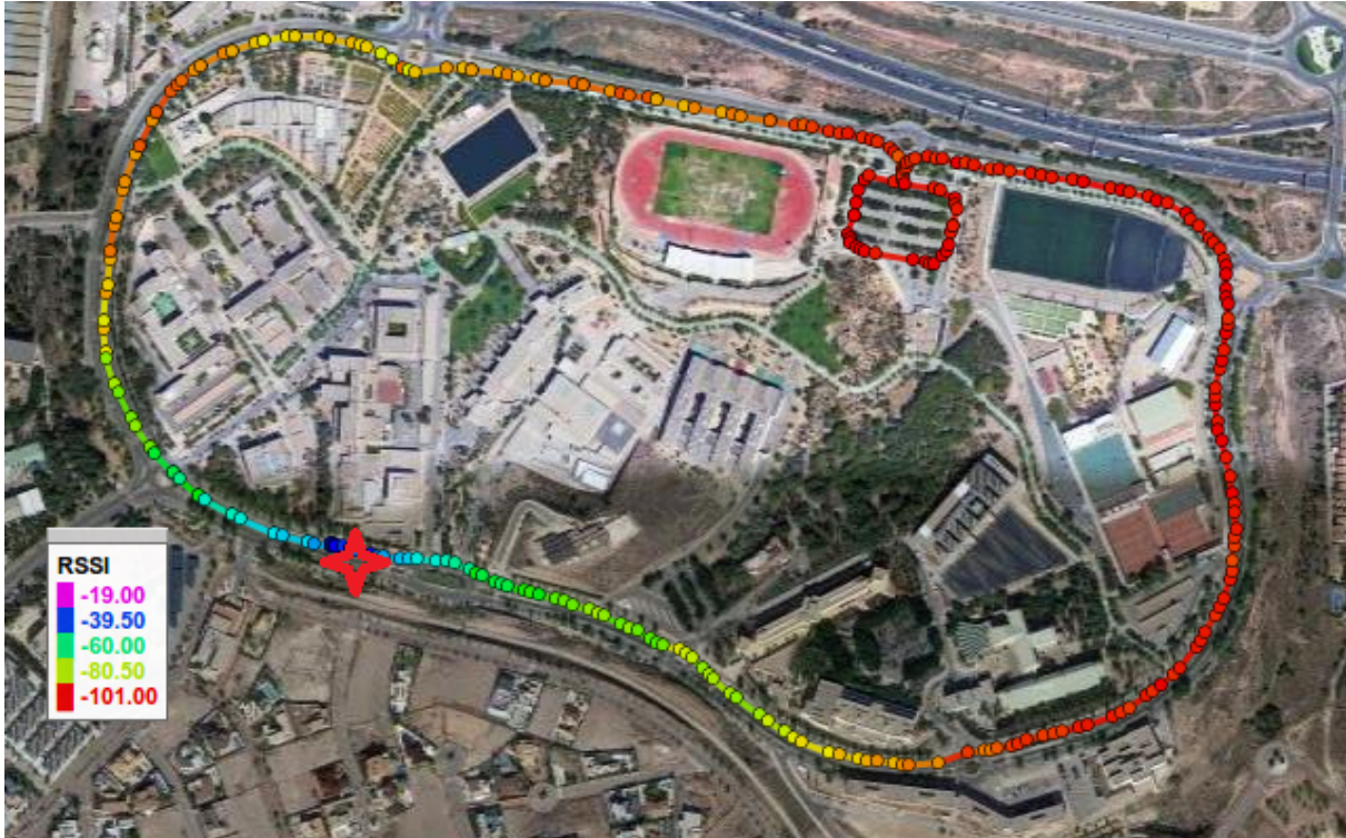
Figure 5: Heat map representing the level of RSSI received by the moving vehicle in the V2V scenario within the university campus. The red star represents the stopped vehicle.
