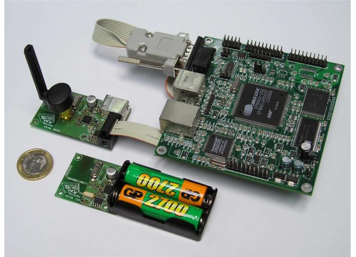
Fig. 7. Developed Active Tag and Reader
