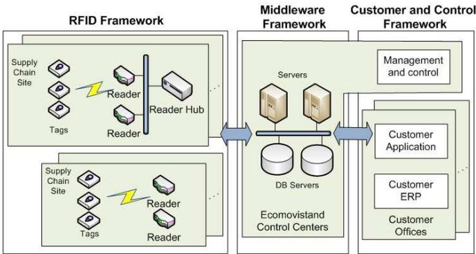
Fig. 5. MEGASTAND frameworks and their physical mapping. RFID Framework components are located in supply chain sites; Middleware Framework components are located in ECOMOVISTAND Control center; C & C Framework has two types of applications: those customer-related running on equipment in customer offices, and those control-related which are in Ecomovistand Control Center. Blue arrows represent typically Wide Area Network communications between components.
