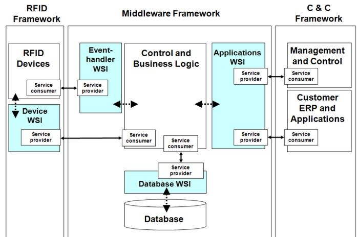
Fig. 6. MEGASTAND Web Services Interfaces. Solid arrows indicate Web Services provision/consumption. Notice that RFID Devices provide control functionality via Device WSI, whereas consume middleware functionality via Event-handler WSI. Dotted arrows indicate no WSI interaction.
