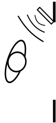
Fig. 3. A single antenna at the door jamb. Depending on user orientation, his body may block the RF signal.
