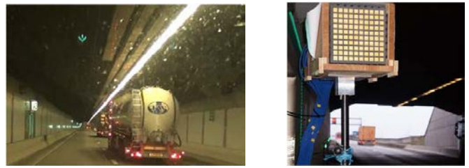
Fig. 1. a) Photo of the tunnel, b) Massive array situated near the exit of the tunnel
