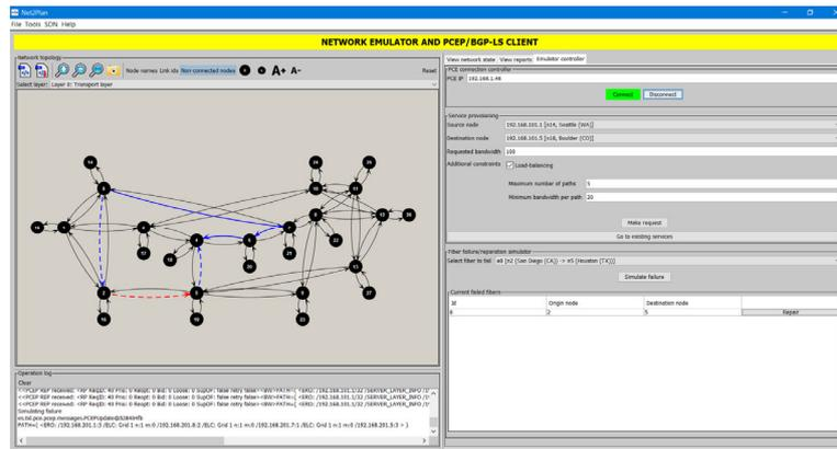
Figure 4. Lightpath rerouting upon fiber failure.
